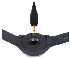
**3** Plug the USB cable into a power source to turn onthe device (*Charging the Device, page 11*).
