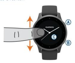
(A) Action button: Press to turn on the device. Press to start and stop the activity timer.
