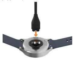
3 Plug the USB cable into a power source to turn on the device (*Charging the Device, page 12*).
